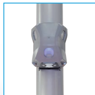
Motion Sensor triggers up to 10 devices. Detects pedestrians, cyclists and cars range (range: 2.5 -75 mph) Range: up to 15m on each side, 9m front and 3m behind at a mounting height of 5m (max).
